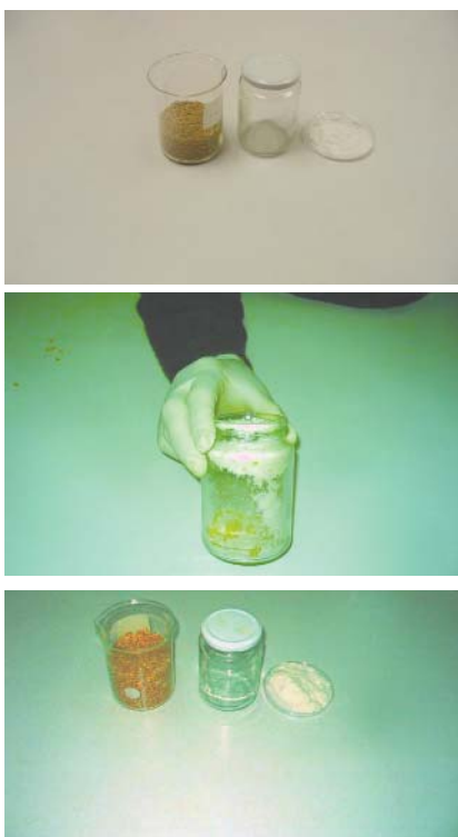
Figure 20. Moisture determination using salt method: equipment (top), dry seed (middle) and moist seed (bottom)
