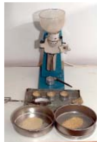
8.10 Grinder and other equipment for moisture test
