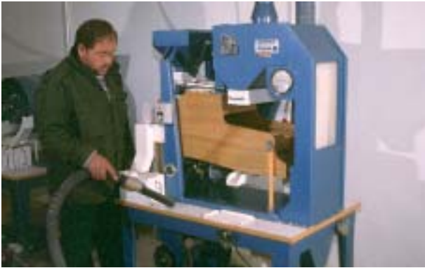
4.3 Air-screen cleaner with three layers
