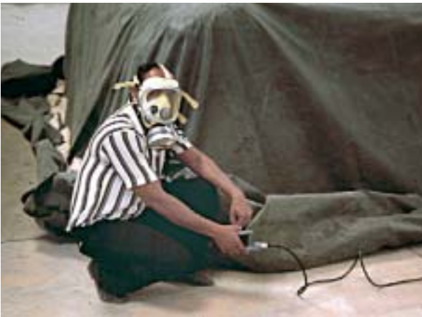
7.5 Measuring phostoxin concentration during fumigation
